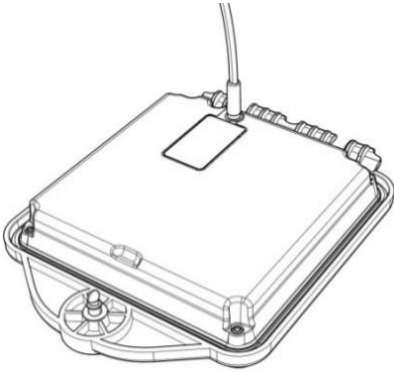
Figure 4.13 Charging the transmitter Li-Ion battery pack
