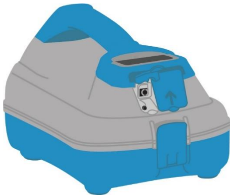
Figure 9.7: Transmitter DC Input
