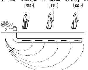
Figure 7.7: Current readings using transmitter signals
