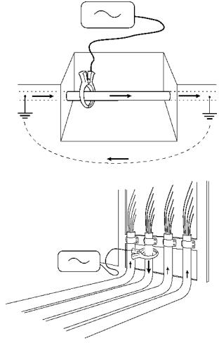
Figures 12.4 – 12.5: Connecting transmitter clamps
