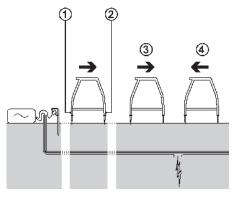
Figure 9.1: Cable sheath fault-finding
