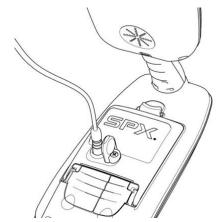
Figure 4.12 Charging the locator Li-ion battery pack
