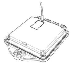
Figure 4.13 Charging the transmitter Li-lon battery pack
