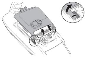
Figure 4.4 Press the retaining latch inwards
