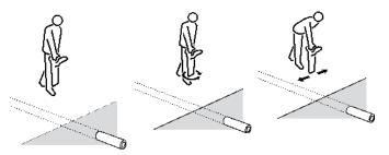
Figure 5.6: Pinpointing a target line
