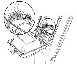
Figure 4.2 Li-ion battery pack connection
