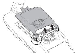
Figure 4.6 installing a new battery pack
