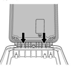
Figure 4.11: Line up the battery pack and press into position
